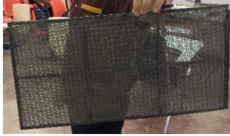
Figure 9. Air filter of air conditioner which lack of cleaning and maintenance.
