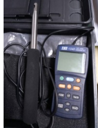
Figure 3. Hot wire type anemometer.
