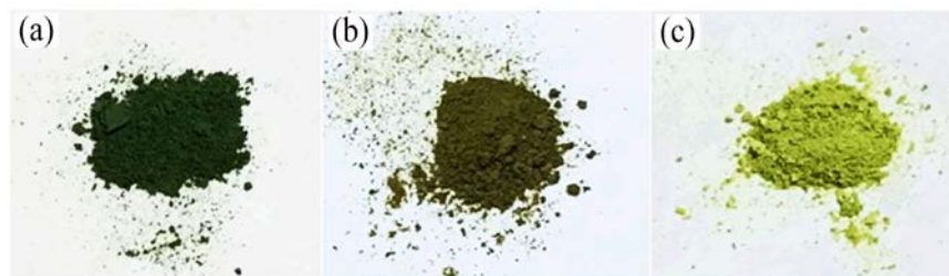
Figure 4. Colors of Co(8hq) 2 (a), MCM_Co(8hq) 2 (b) and MCMCo(II)_8hq (c)
