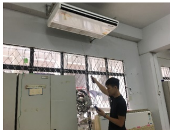
Figure 7. Air velocities measurement.
